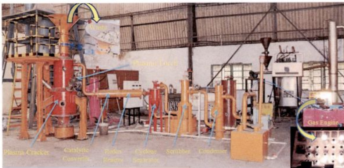
Fig 5.7: Plastic Disposal Unit at CSIR-CMERI (Capacity: 25 kg/ hr)
