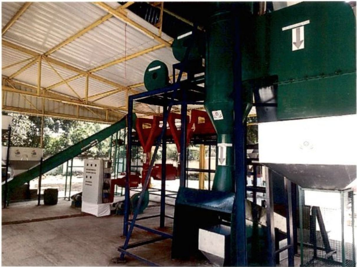
Fig 5.3: Mechanized Segregation Unit for Live Waste at CSIR-CMERI (Capacity: 50 kg/h)
