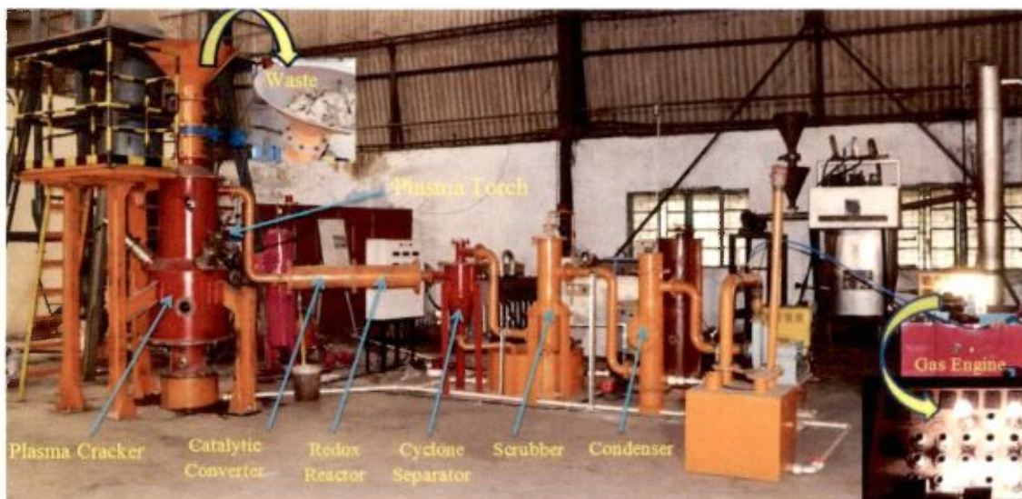
Fig 5.7: Plastic Disposal Unit at CSIR-CMERI (Capacity: 25 kg/hr)
