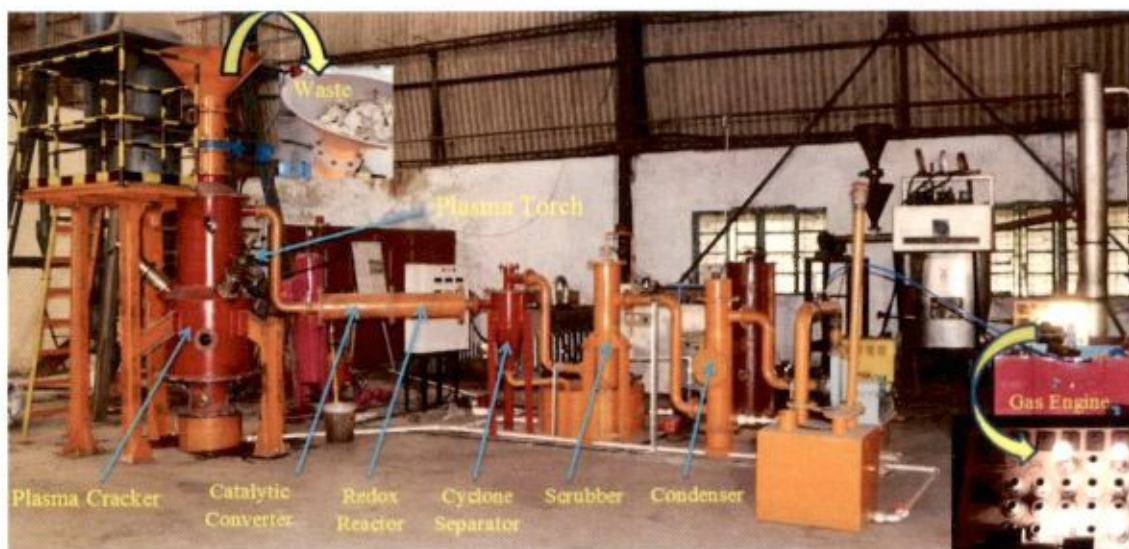
Fig 5.7: Plastic Disposal Unit at CSIR-CMERI (Capacity: 25 kg/hr)
