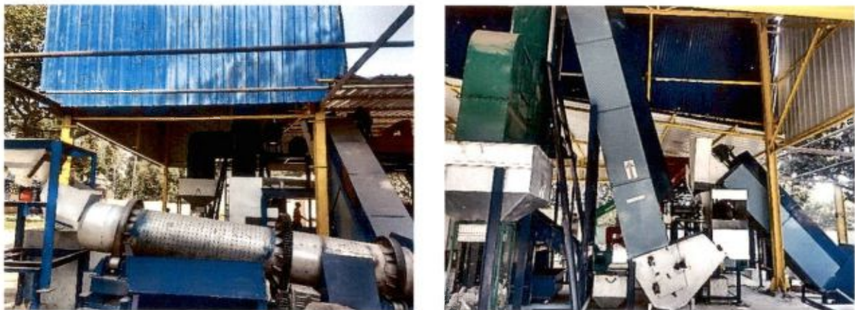
Fig 5.5: Mechanized Segregation Unit for Dead Waste at CSIR-CMERI (Capacity: 100 kg/h)
