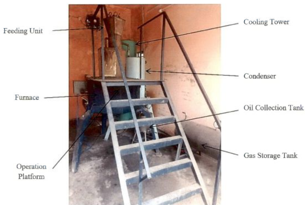
Fig 5.9: Polymer Waste Pyrolysis Unit at CSIR-CMERI (Capacity: 20 kg/ batch)
