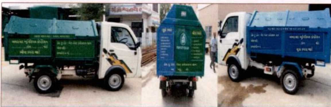
Figure 72 The new vehicle, for waste collection, introduced by AMC with closed body having different compartments with tipping agreement for collection of segregated waste from citizens
